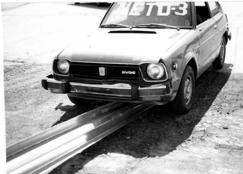
FIGURE 28. System Configuration and Impact Location for NETD-3.
